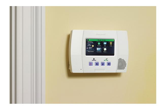
This wireless system can be removed and re-installed at will. Moving the unit from one vacant home to the next can spread the cost out significantly. Changes would be made at the Central Station, so they would know where the building was and who to contact if the building was entered illegally.
